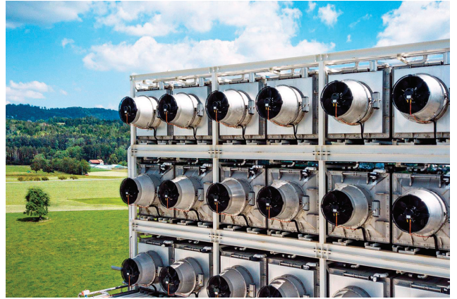
At this commercial direct air capture plant in Hinwil, Switzerland, fans draw in air and chemicals help bind the carbon dioxide so it can be stored underground. Credit: Climeworks.
