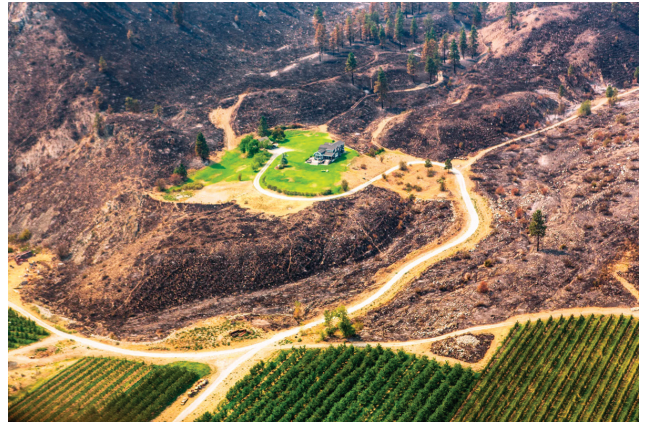
This home survived the otherwise devastating Wolverine Fire outside of Chelan, Washington in 2015 thanks to firescaping with native plants.
