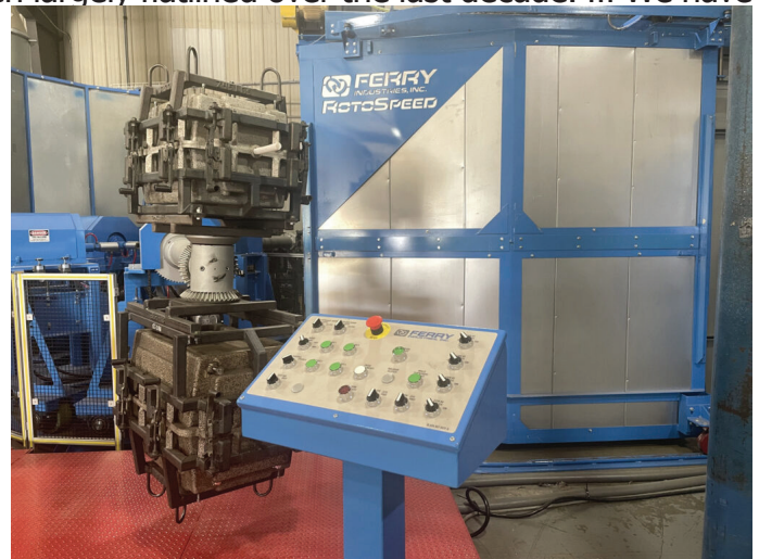
Ruff Land Kennels of Tea, S.D., uses high-tech machines to rotationally mold its industry-leading one-piece kennels for pets.
