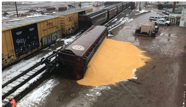
Six box cars carrying grain derailed under the 10th Street Bridge in downtown Sioux Falls in March 2018, an accident caused when the rail lines were found to be too far apart, according to federal reports. Photo: Courtesy Argus Leader
