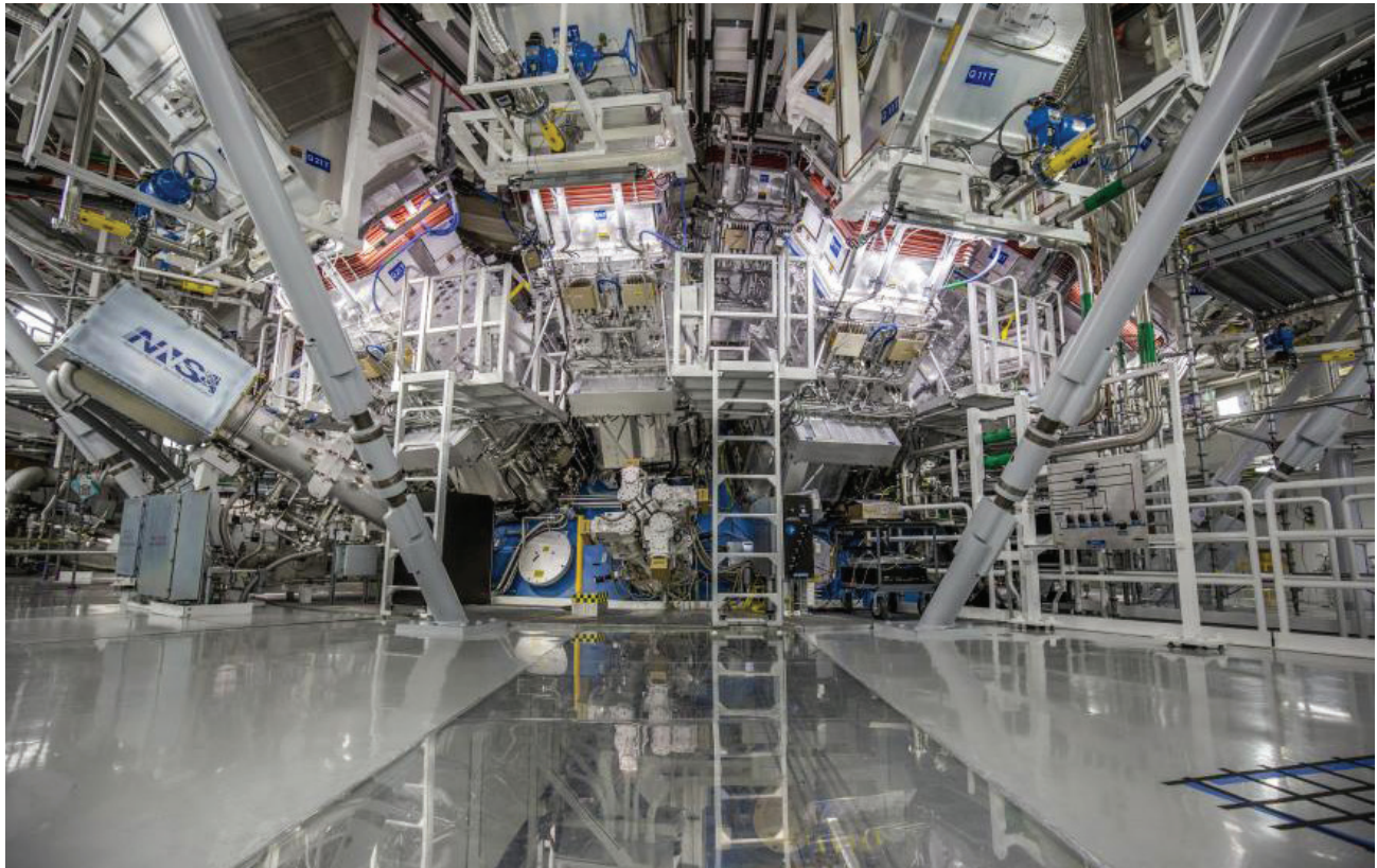
The target chamber of Lawrence Livermore National Laboratory's National Ignition Facility, where 192 laser beams delivered more than 2 million joules of ultraviolet energy to a tiny fuel pellet to create fusion ignition on Dec. 5, 2022. (Lawrence Livermore National Laboratory)
