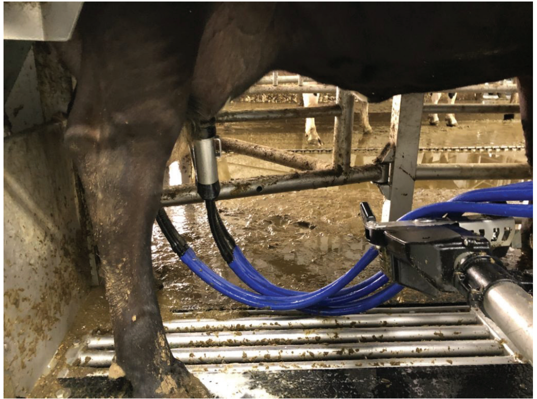
This cow is undergoing milking performed by a robotic arm and milking machine at the Drumgoon Dairy. The robotic arm contains a high-definition camera that locates each teat and cleans it before attaching milking cups. Photo: Bart Pfankuch, South Dakota News Watch
