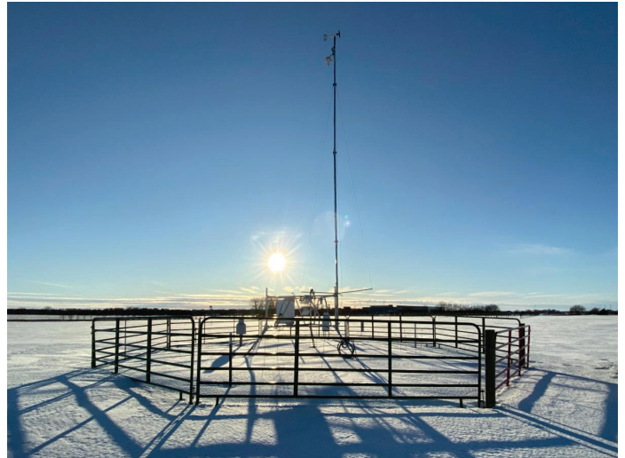
The South Dakota Mesonet weather station on the SDSU campus in Brookings, S.D., is the first of 500 stations upgraded to conduct enhanced soil moisture and snow monitoring to provide crucial data about snowpack levels and flood risk.
