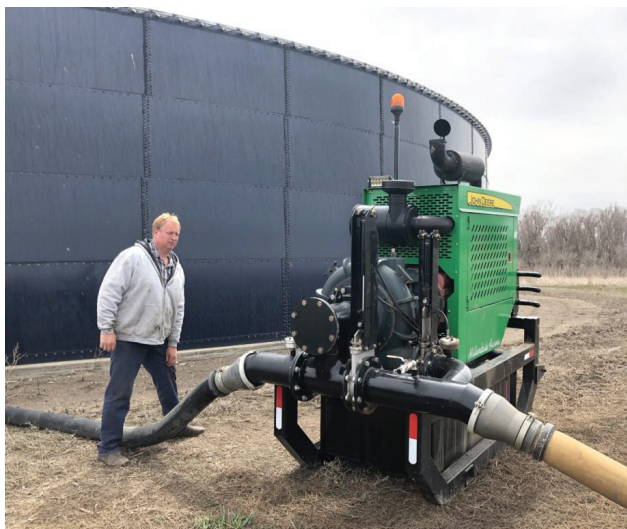
During spreading operations, farmer Matt Moeller checks a pump that is part of a mechanical system that stirs the manure and then pumps it into a pipe that will carry it to nearby farm fields.
