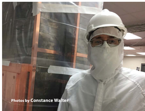
Left: Vince Guisepppe stands next to an extra lead brick monolith, which keeps the shield sealed if a working module needs to be removed for service. Right: Jared Thompson stands in front of the completed shield. The shield team is encasing the poly shield in aluminum as a fire suppression element.
