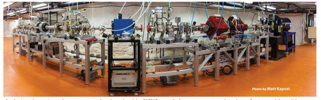
Accelerators rely on an ion or plasma source to produce charged particles. CASPAR uses radio-frequency energy to produce a beam of protons or alpha particles from hydrogen or helium gas. The electric field speeds up the beam of particles, which are steered and focused with magnets through the beam pipe in a vacuum. A 25-degree bending magnet ensures that only particles with the right energy are directed to the target.
