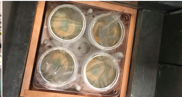
Left: Photomultiplier tubes are placed into a low-background counter. Right: PMTs sit near a germanium crystal surrounded by copper and lead shielding.
