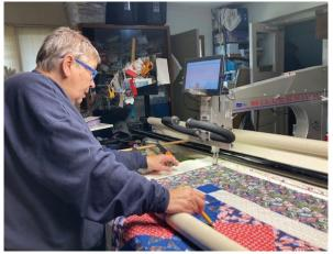
Karen Wolter guides the guilt top through the machine. A computer is connected to the quilting machine to tell the machine which pattern she has chosen. (Photo by Dorene Nelson)
